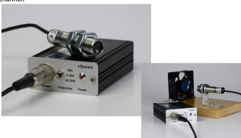
At the same time, the impulses coming from the LED sensor are output to a TTL output.
